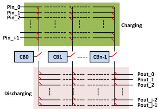
Figure 2. Charging and discharging networks.
