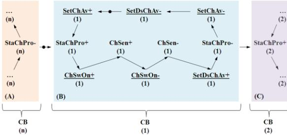
Figure 3. FIFO PDU charge control, (underlined signals are inputs).
