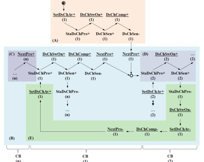
Figure 4. FIFO PDU discharge control. (A) starting from CB(1) after initialization; (B) steady-state; (C) CB(n); (D) CB(2); (E) power continuity provision.
